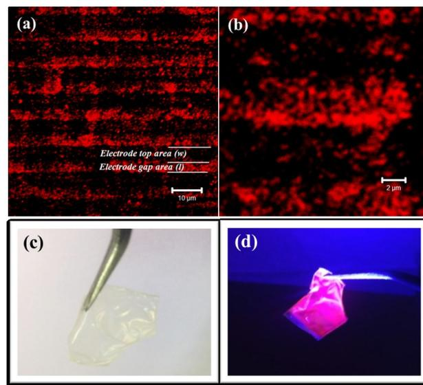
**Figure 6.** (a-b) High magnification confocal fluorescence microscope images of functional film on IPS substrate. The film detached from the IPS substrate (c) under normal and (d) UV light.
