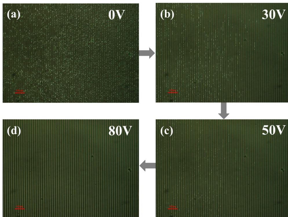
**Figure 3.** Optical microscope images of RM/QRs mixture after coating on IPS substrate (a) without any applied voltage and (b)-(d) with gradually increasing voltage. (Scale- 100  $\mu\text{m}$ )
