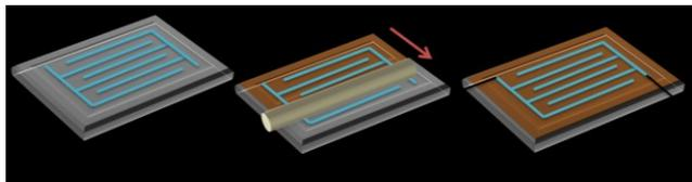
**Figure 2.** Pictorial depiction of method followed to prepare QRs functional film (a) IPS substrate (b) RM/QR mixture coating with shearing bar. (c) RM/QR mixture on IPS substrate under applied in-plane ac square field and illuminated with UV light.
