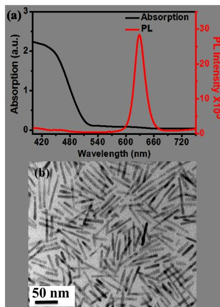
Figure 1. (a) Absorption and PL emission spectra of CdSe/CdS QRs and (b) corresponding TEM image.
