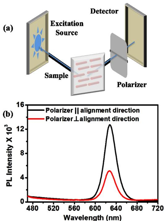
**Figure 5.** PL measurement (a) Experimental setup for measuring the PL (b) PL spectra measured from functional film with polarizer position parallel and perpendicular to the alignment direction.
