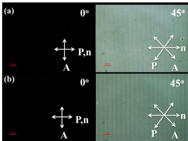
**Figure 4.** POM Images of film under cross polarizer. (a) RM/QRs mixture on IPS substrate under applied electric field before UV curing and (b) after UV curing (Scale-100  $\mu\text{m}$ ). n represents the alignment direction of RM.
